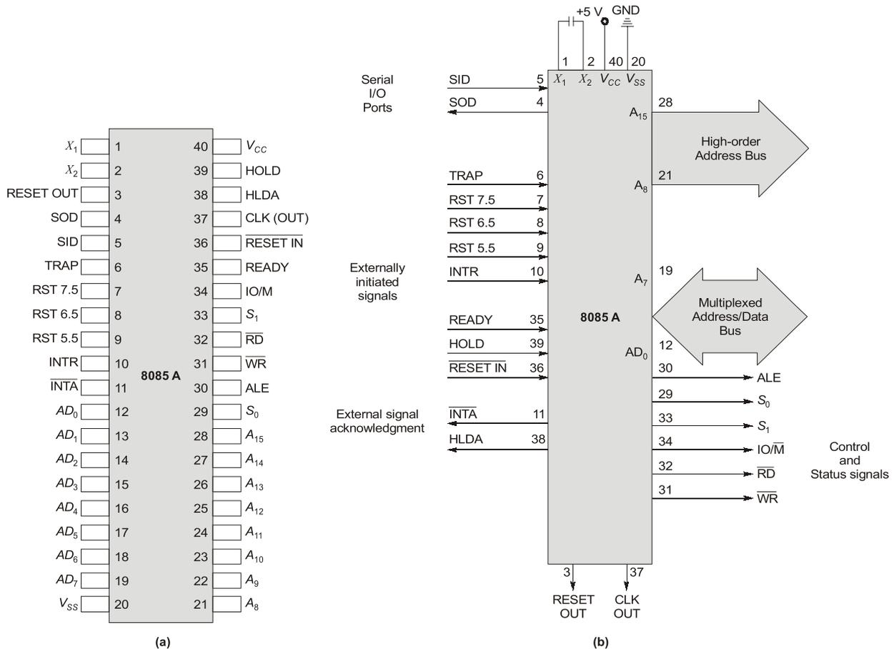
Figure-1.2: 8085 Pinout
